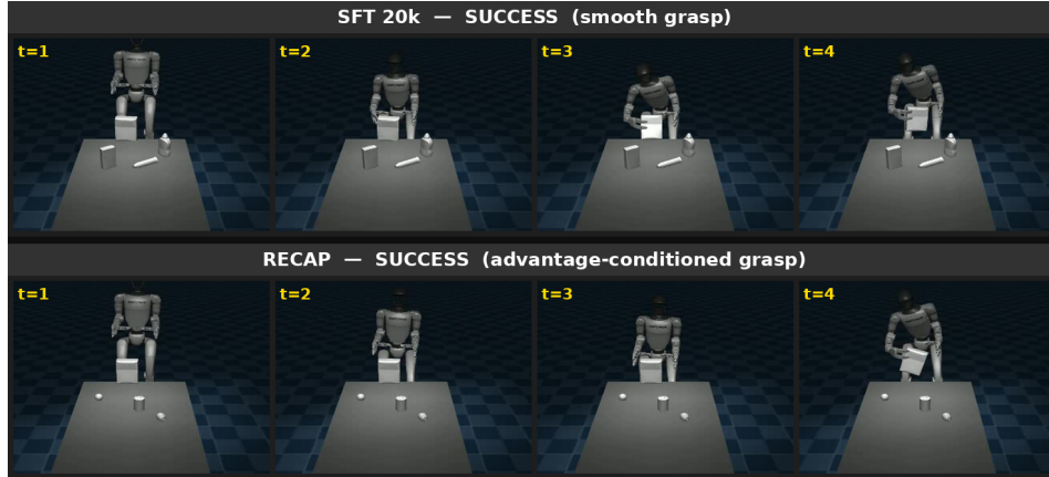
Figure 3: Qualitative comparison of SFT and RECAP grasping behavior on BendPickMP. Top: SFT@20k successful grasp (episode 383, 176 steps). Bottom: RECAP advantage-conditioned successful grasp (episode 013, 142 steps). Frames sampled from the grasp phase (30–98% of episode).
