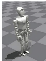
(a) Robot policies trained without environmental projectiles walk with larger yet less stable strides by standing straighter
