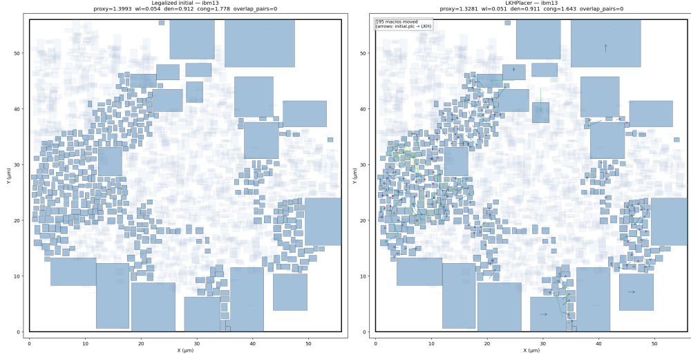
Figure 3: ibm13, legalized analytical seed (left) versus refined output (right). Arrows show macro displacement, with color proportional to move distance. Both placements are overlap-free and the proxy cost improves over the run. The values shown are from a development run and differ slightly from the final per-design results in Figure 2.
