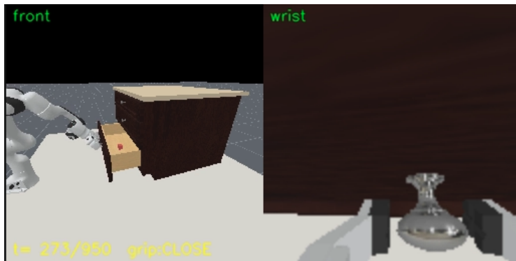
Figure 2: The DrawerCubeTakeOut task in SAPIEN/ManiSkill: a Franka Panda faces a three-drawer cabinet with a cube hidden in one (randomized) drawer layer.
