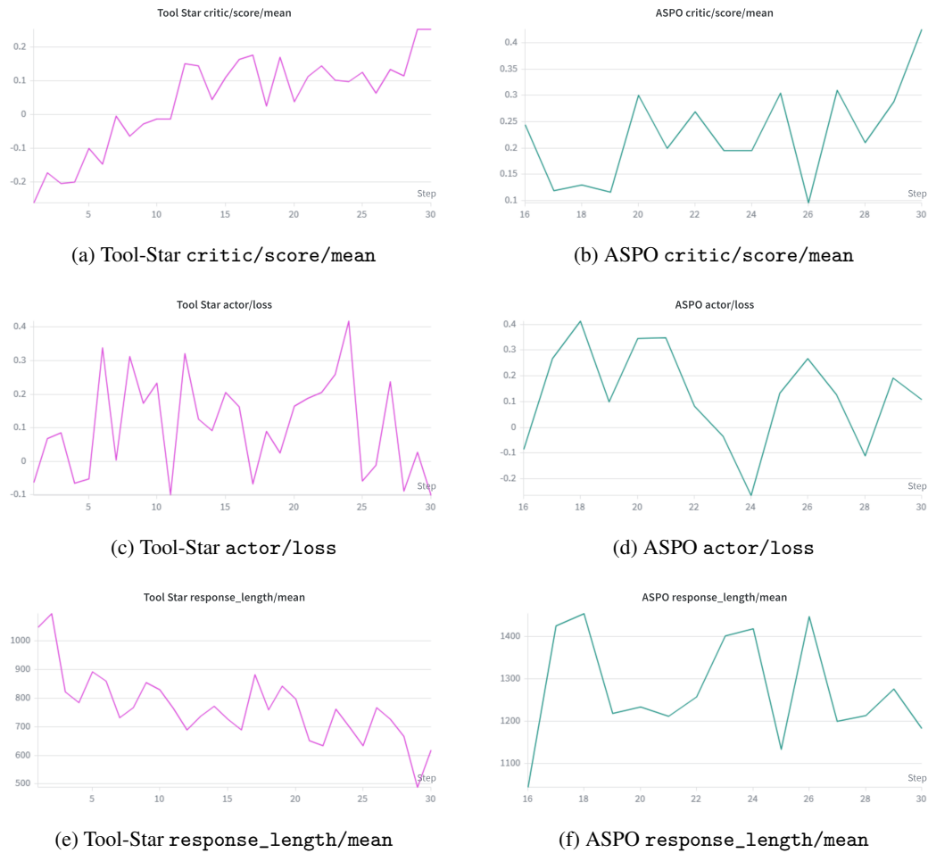
Figure 8: Training-time telemetry for the matched-compute runs. Left: Tool-Star GRPO baseline (steps 1–30). Right: our ASPO run (steps 16–30). Rows: critic/score/mean, actor/loss, and response_length/mean.
