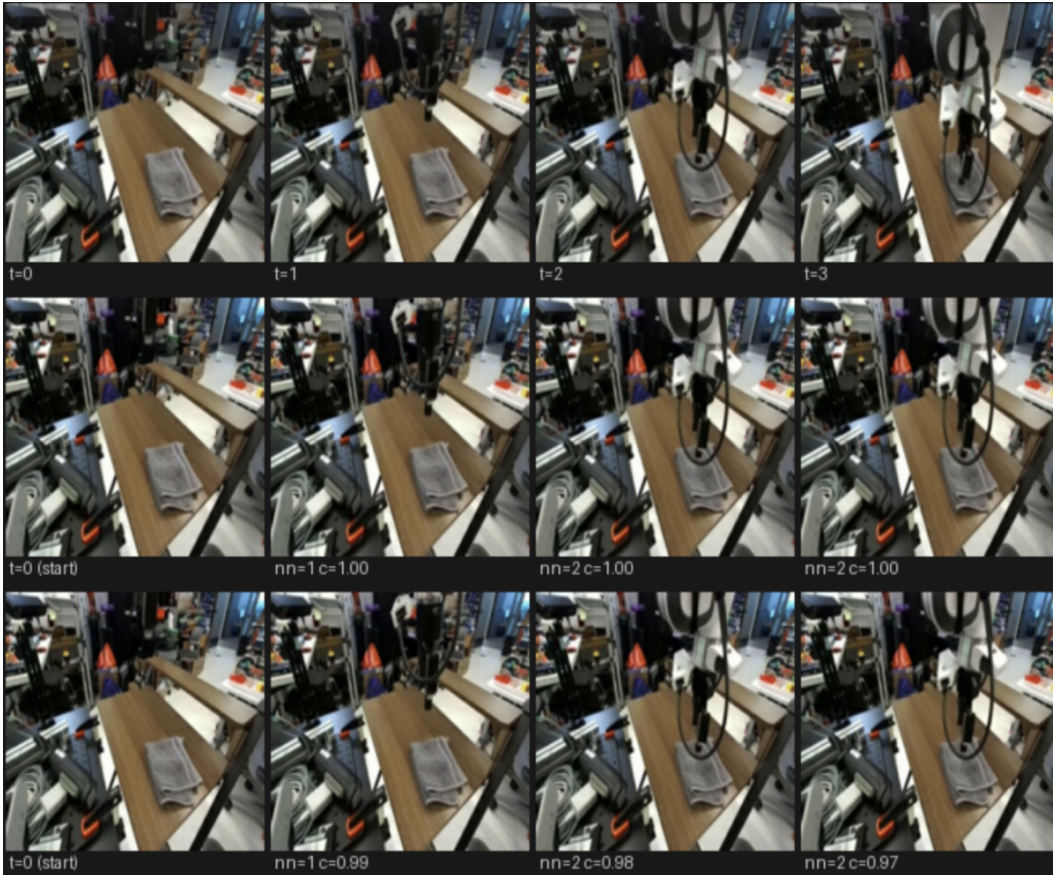
Figure 2: Rollout comparison on a DROID episode. Row 1: Real robot frames ( t = 0 \dots 3 ). Row 2: IDM-driven world model rollout (upper bound, confidence c = 1.00 ), which has access to real future frames. Row 3: Controller-driven rollout (confidence c = 0.99 \rightarrow 0.97 ), using only real robot actions with no future frame access. The controller trajectory closely tracks the IDM upper bound.
