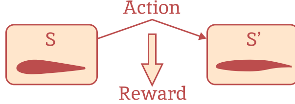
Figure 4: State-Action-Reward diagram for the deep RL based shape optimization procedure.
